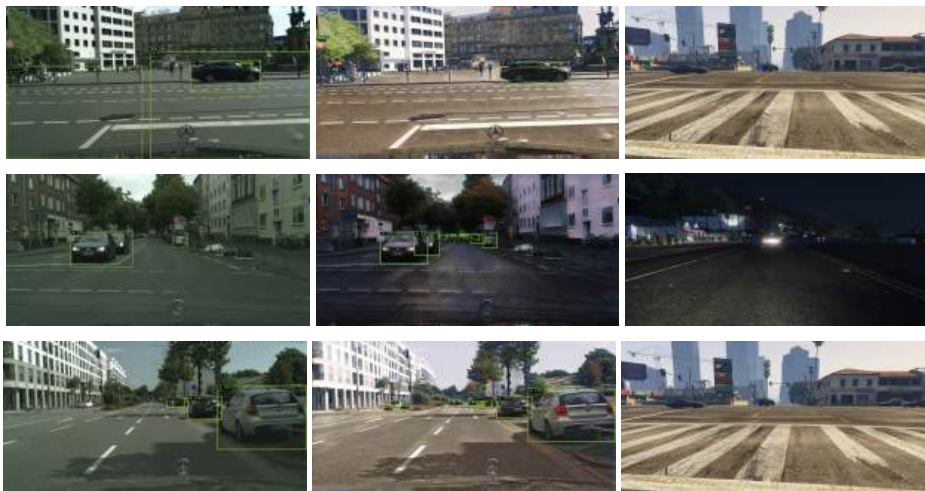
Figure S3: The Sim10k \rightarrow Cityscapes adaptation scenario. In all cases the detector model is trained on the Sim10k dataset and evaluated on Cityscapes. We visualise detection inference results on Cityscapes (column 1), inference result on the translated image (column 2) and an (unpaired) real image from the Sim10k dataset, to aid effective translation assessment (column 3).
